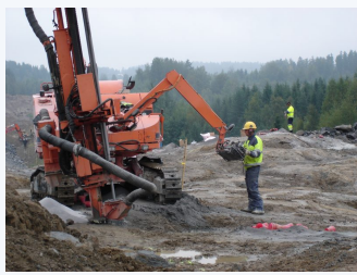
Foreuse (Drill rig) Blasthole drill
